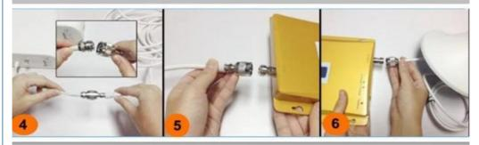
Connect indoor antenna to the booster "Mobile" side by cable. (Outdoor antenna to the booster "BTS" side.)
